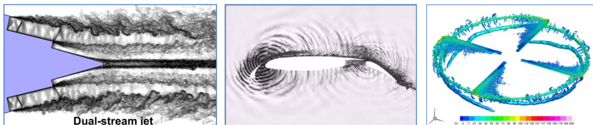
Figure 1: Instantaneous flow fields: dual-stream jet (left), acoustic radiation by 30P30N HLD configuration (middle), vortical flow generated by helicopter rotor at hover mode (right).
